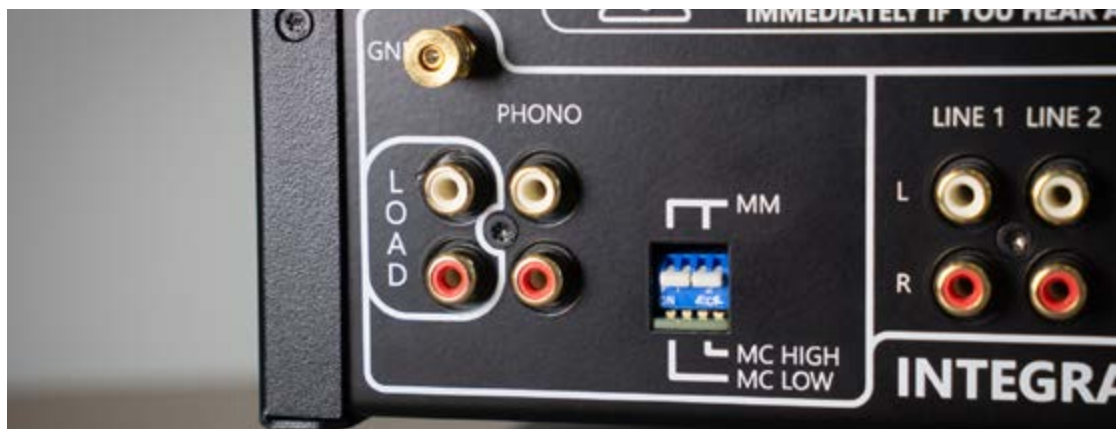
Internal phono stage caters for MM and MC inputs (right sockets) offering gain at 48/60/70dB, with bespoke MC loading options via external plugs (left sockets)
