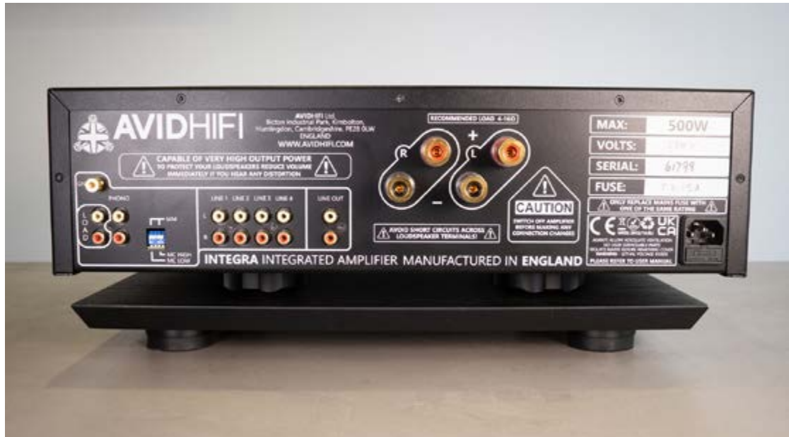
Rear panel socketry includes RCA in/outs (no XLR) plus AVID's own gold plated speaker cable binding posts
