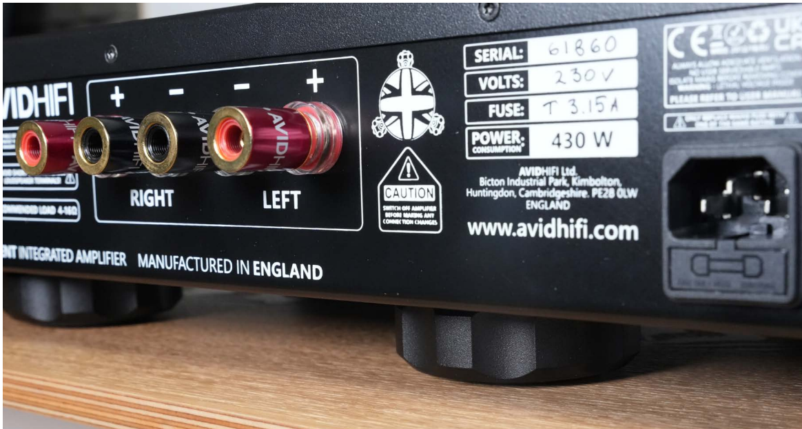
A window into the Accent's build quality, showing its bespoke speaker sockets and oversized metal feet for superior stability
