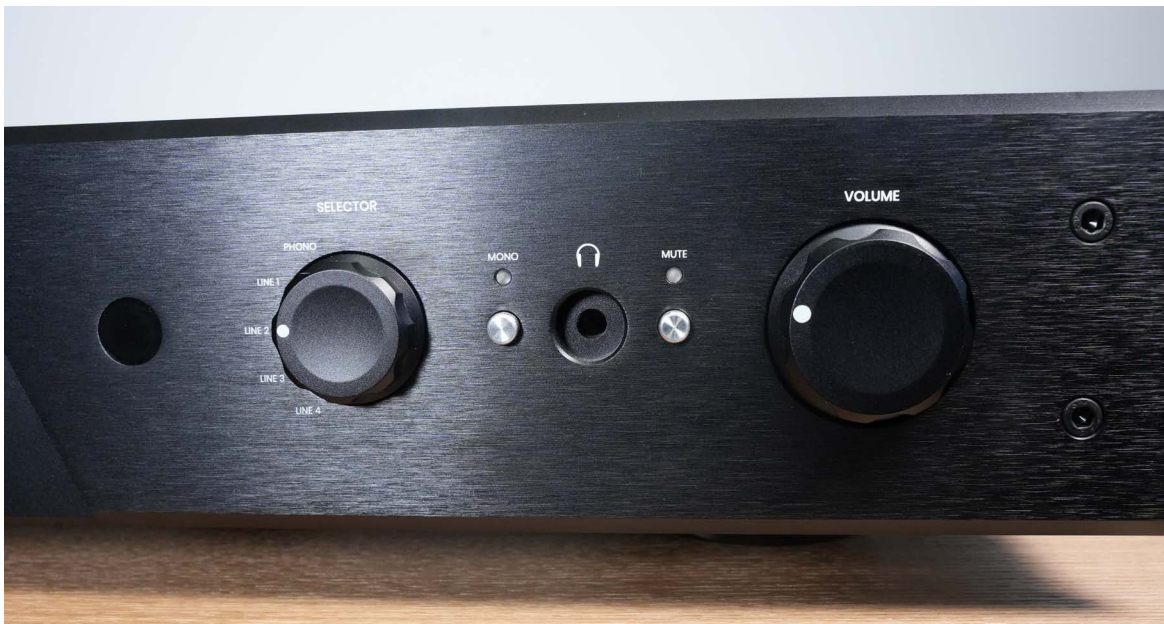
Front panel controls are limited to volume, input selection, mute and mono mode. On/off switch? That's hidden underneath...
