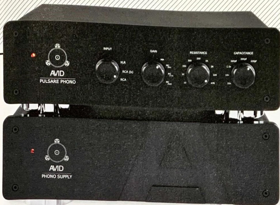
LEFT: While there's no subsonic filter option, the Pulsare is equipped with a huge range of input loading and gain settings to accommodate almost any choice of pick-up
